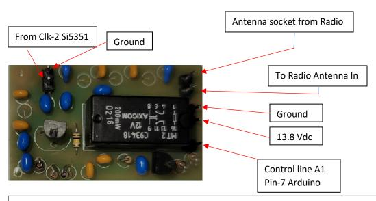
Note: Use a good quality coax such as RG-174 or equivalent from Clk-2 of the Si5351 to the HF RX.
